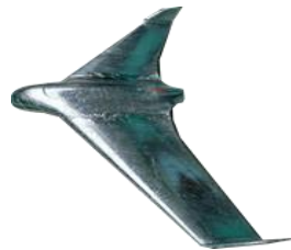
Figure 1. Application of aluminum foil on Skywalker X8 UAV to shield electromagnetic interference
