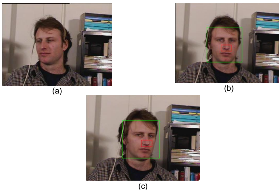
Figure 5. (a) A sample frame from jam7 data, (b) Detected nose and face using Haar classifier, (c) Tracking of previously detected objects (Source: Cascia et al)
