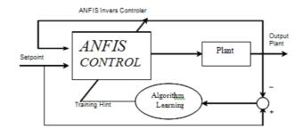
Figure 3. Block diagram control of ANFIS
