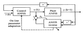
Figure 4. Block diagram control of ANFIS on closed house for broilers
