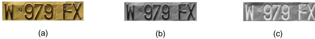
Figure 9. The inverted grayscale image of public transportation license plate, (a). yellow license plate, (b). grayscale image, (c). inverse image
