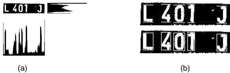
Figure 13. The optical character recognition, (a). Valley (space) horizontal and vertical projection, (b). result of segmentation
