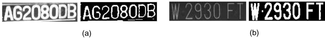
Figure 10. The dilation morphological process, (a). large character and its erosion result, (b) small character and its dilation result
