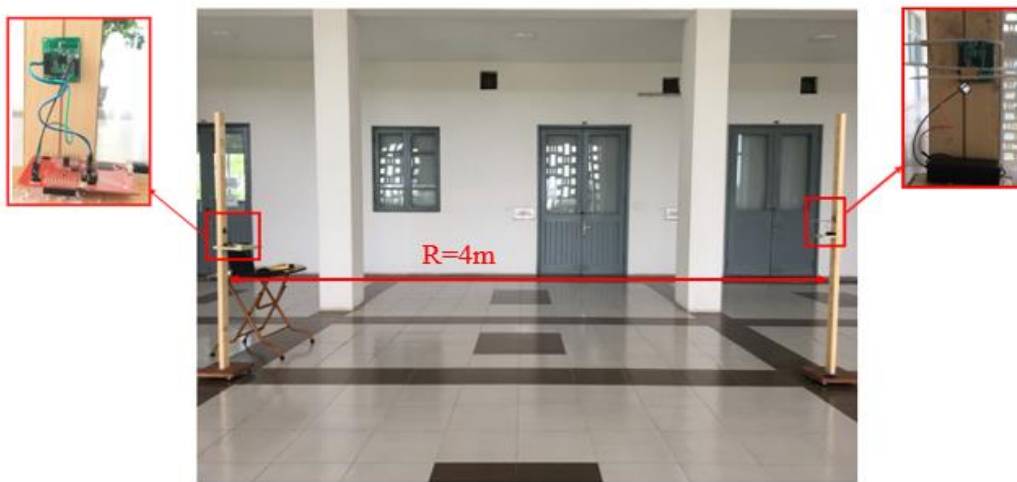
Figure 6. Gain measurement scenario of MIFA antenna integrated WSNN
