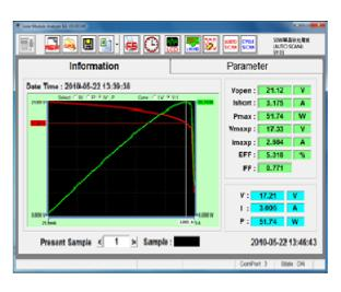
Figure 4. V-I characteristics of a GE 50W solar panel
