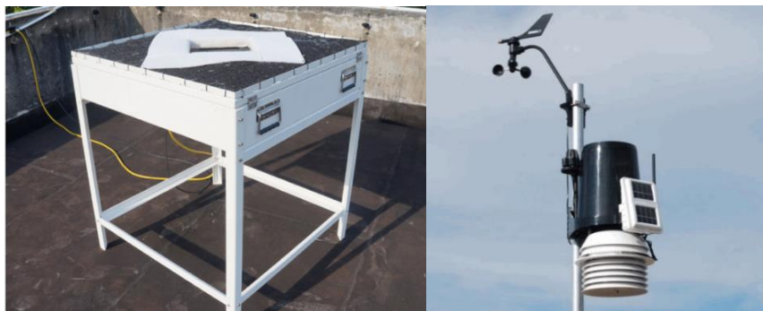
Figure 2. 2-dimensional video disdrometer (2DVD), and the co-located automated weather station installed on the roof of WCRL
