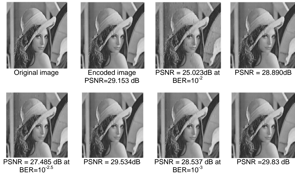
Figure 6. Restored lena image at different BER using median filter. (Left: Degraded. Right: Restored)
