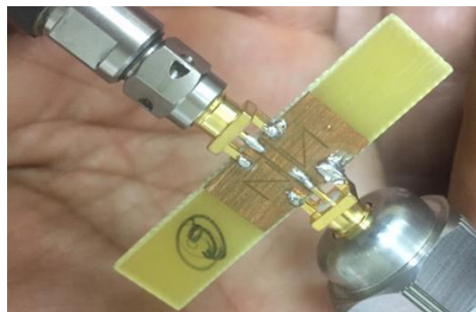
Figure 10. The photograph of the proposed Z-DGS bandstop filter
