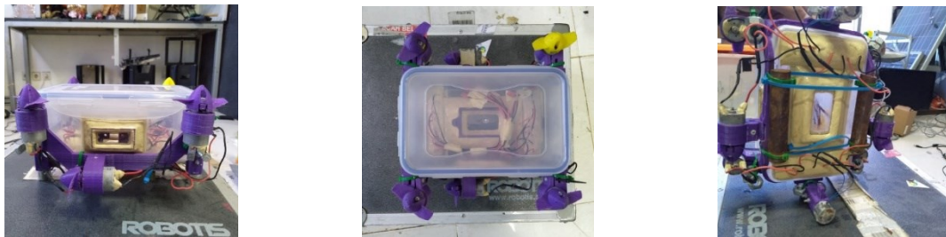
Figure 7. Mechanical assembly of fitoplankton SAS ROV
