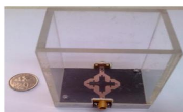
Figure 7. Sensor with acrylic holder for sample loading [63]
