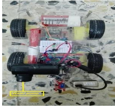
Figure 13. Fire extinguisher system prototype
