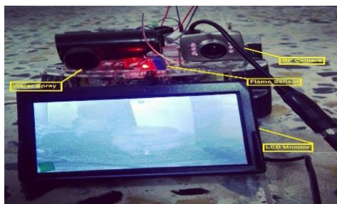
Figure 12. Fire monitoring system prototype
