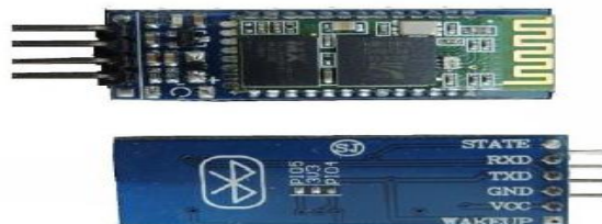
Figure 8. HC-06 bluetooth module
