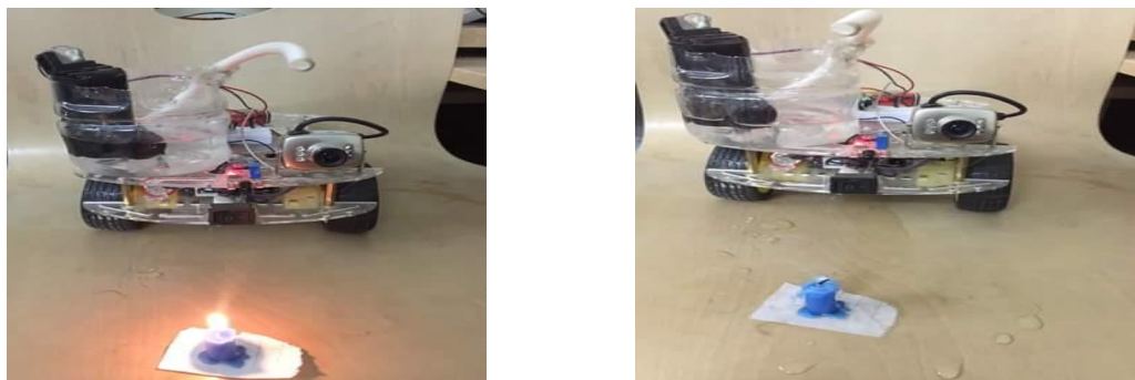
Figure 15. Extinguishing the fire detected by the robot
