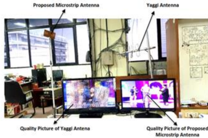
Figure 14. Field measurement of proposed antenna compare with yaggi antenna
