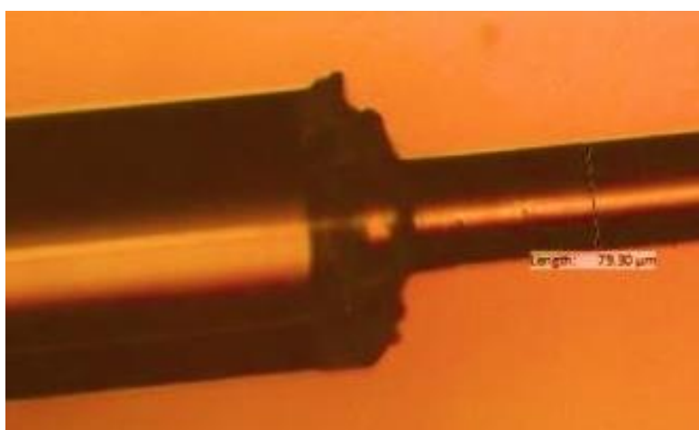
Figure 3. Etching process of fiber optic using HF 40% over 30 minutes
