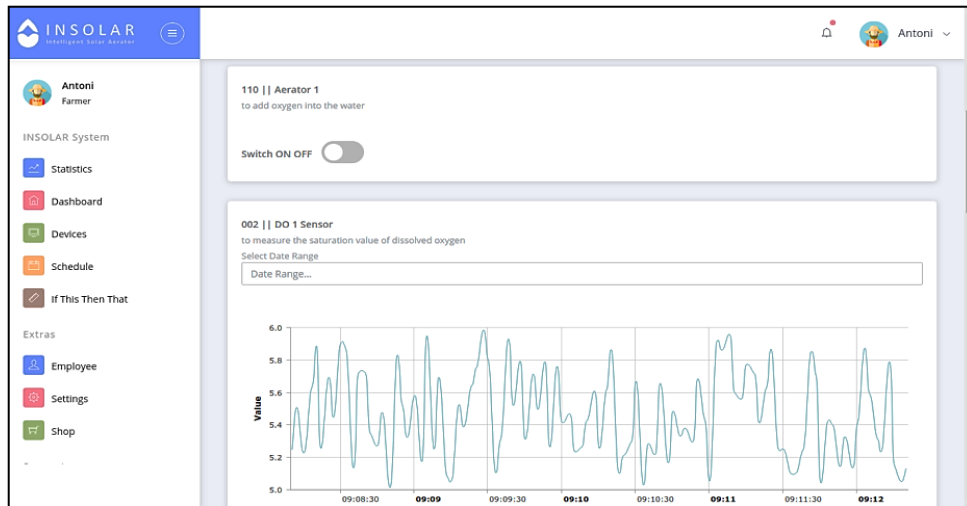
Figure 4. Detail dashboard page show the graph of dissolved oxygen
