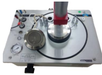
Figure 2. Cylindrical electrode configuration for DS experiment
