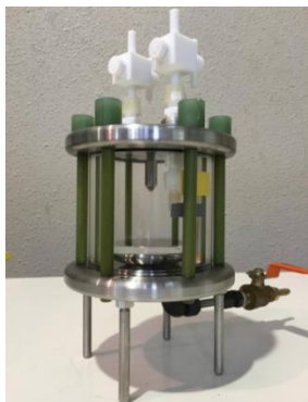
Figure 1. Oil chamber used for PD measurement
