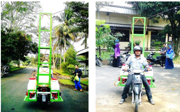
Gambar 7 Mobile sprayer machine (prototipe A) hasil rancangan.
