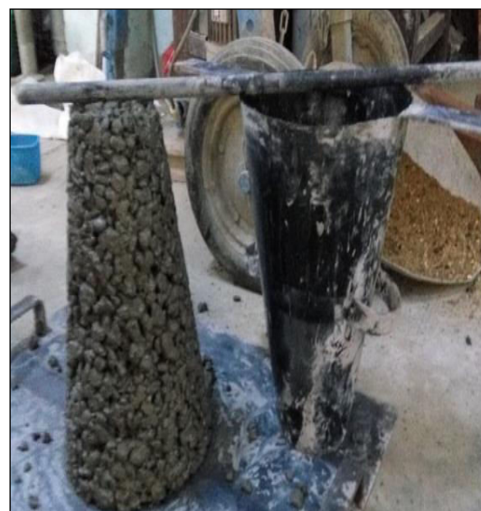
Figure 3. Slump Test of Concrete
