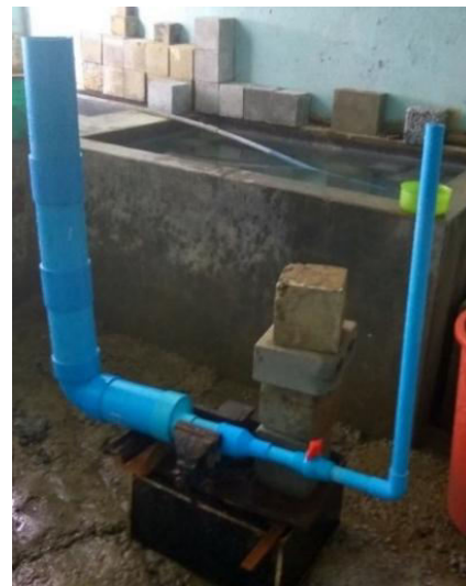
Figure 7. Water Permeability Test
