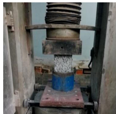
Figure 5. Compressive Strength Test
