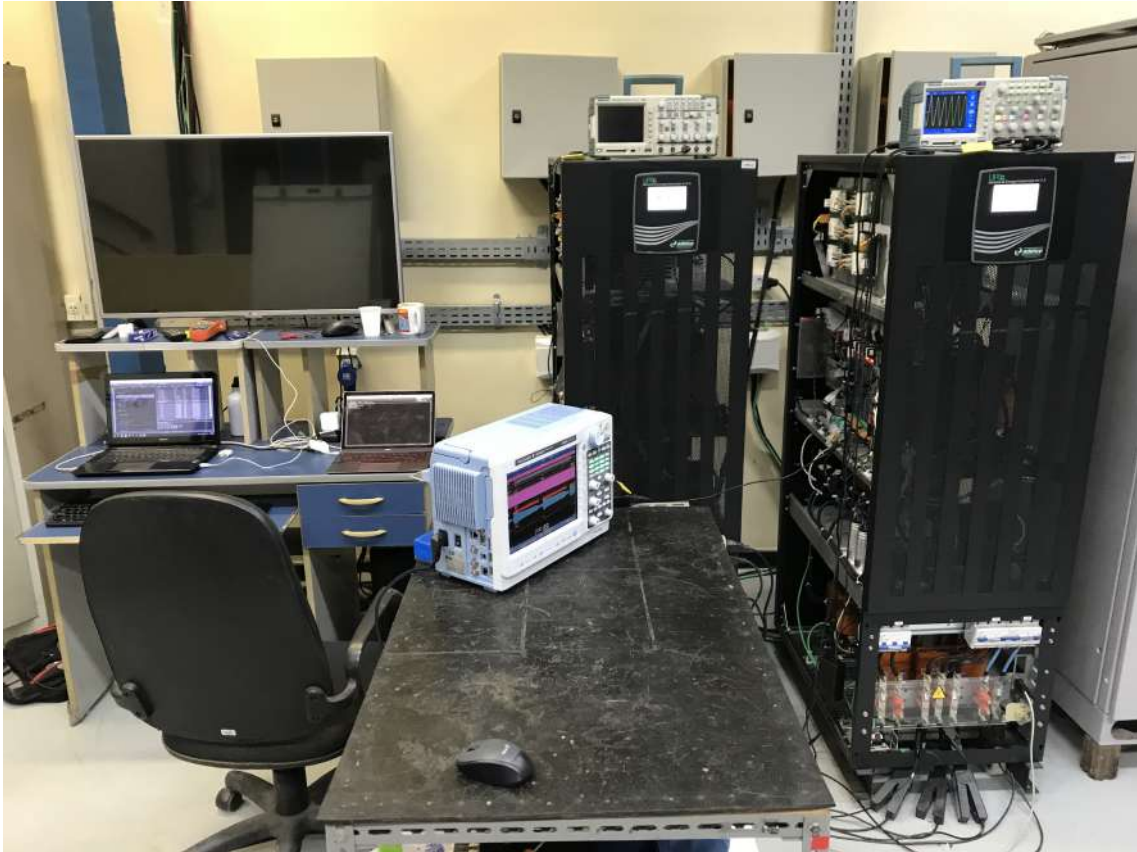
Figure 5.15: Test rig composed of two back-to-back converters connected in parallel. Also in the picture are the computers used for embedded code loading, debugging and supervision, and the oscilloscope used for all shown measurements, a Yokogawa DL850EV .
