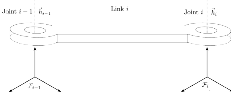
Figure 2.6: Placement of joint i axis for the Jacobian calculation
