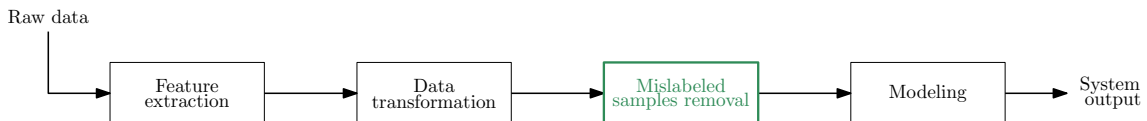
Figure 3.6: Each sample i joins the training set k - 1 times during cross-validation. After each training, the algorithm compares the predicted value during training with its true label; if they are equal, it increments the sample score by one unit. When the training ends, if the score is larger than a given threshold, the respective sample goes to the next block.
