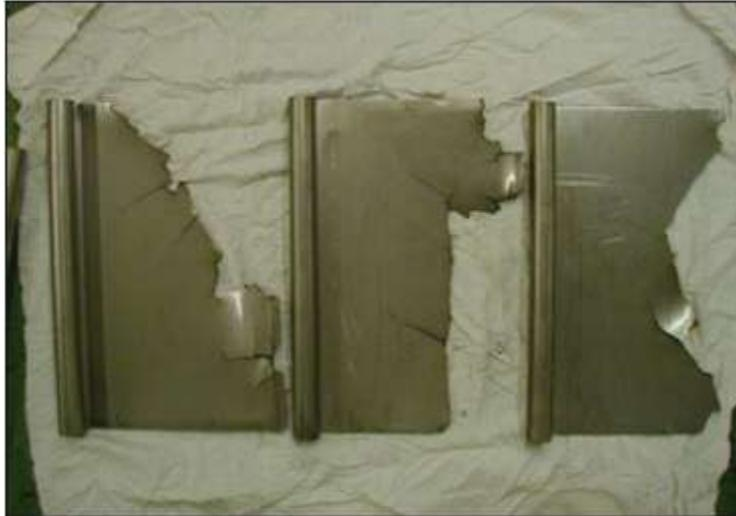
**Figura 3-15: Flap valves quebradas**
