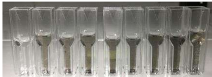
Figure 3.1 - Evolution of a dispersion of 0.33% CNT in water and surfactant after different sonication energies
