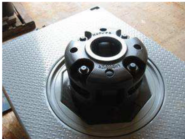
Figura 5 – Bucha do Kelly encaixada na bucha mestre. ( http://hackerinternational.com/images/products/Kelly_Bushing.jpg )
