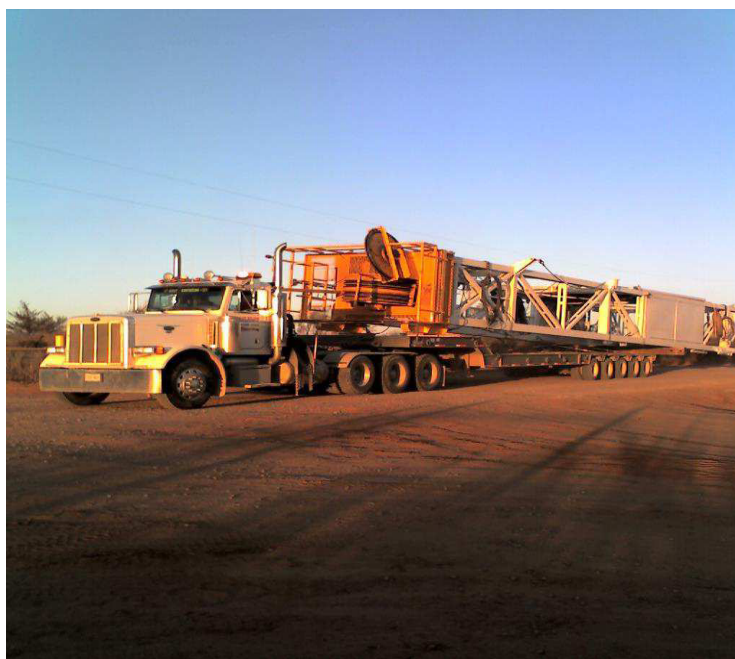
Figura 52 – Caminhão transportando a torre de perfuração ( http://declinemagazine.com/nucleus/rig-moving )
