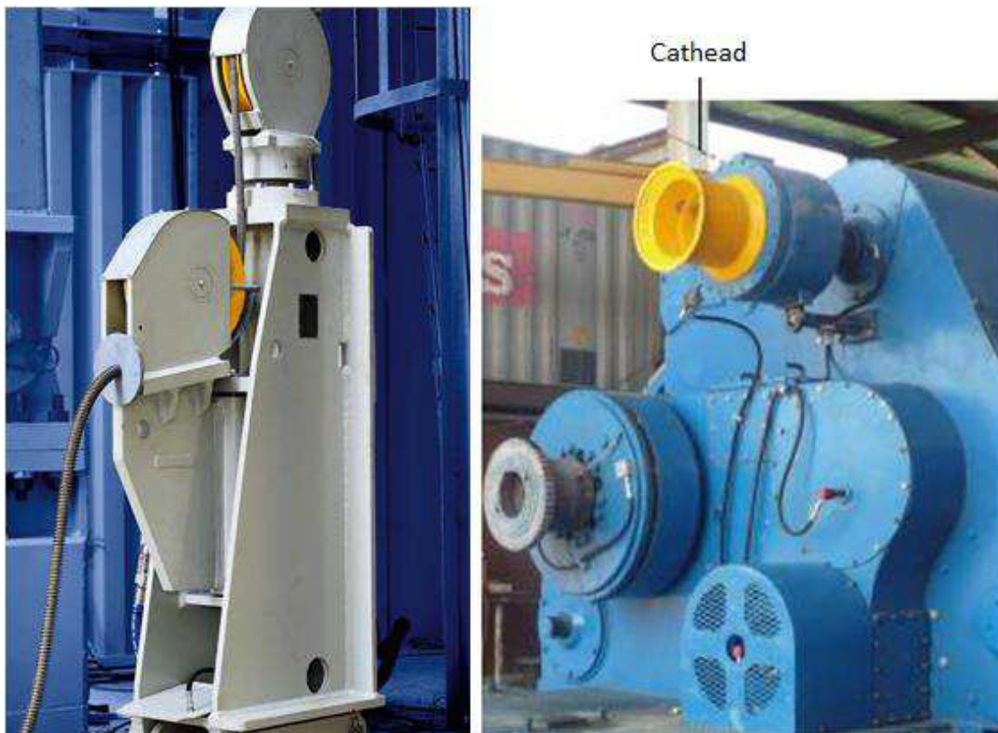
Figura 56 – Cathead hidráulico e cathead do Drawworks ( http://totaldrillingsupply.com/of1017 . e www.seekpart.com )
