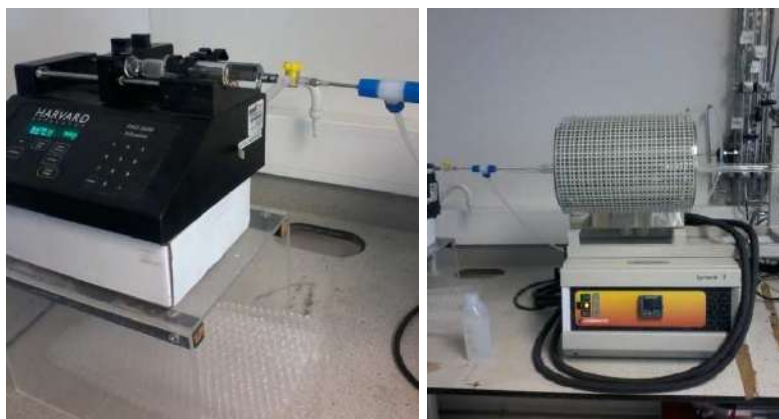
Figure 3.5.1 – Catalytic reaction Unit 2: ethanol feed pump and reactor system.
