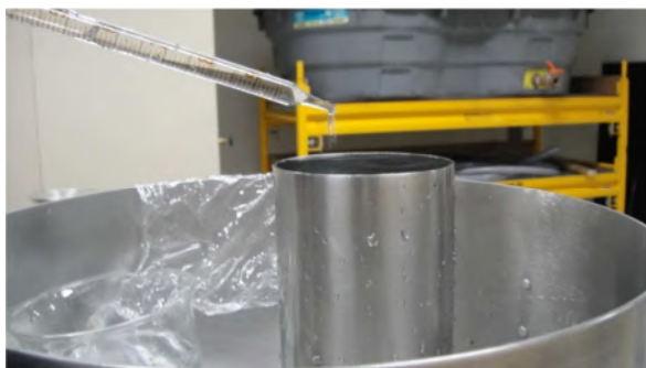
Figure 6. Meniscus adjustment using a pipette.
