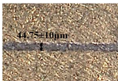
FIG. 12: Detailed image of the interface tin layer
