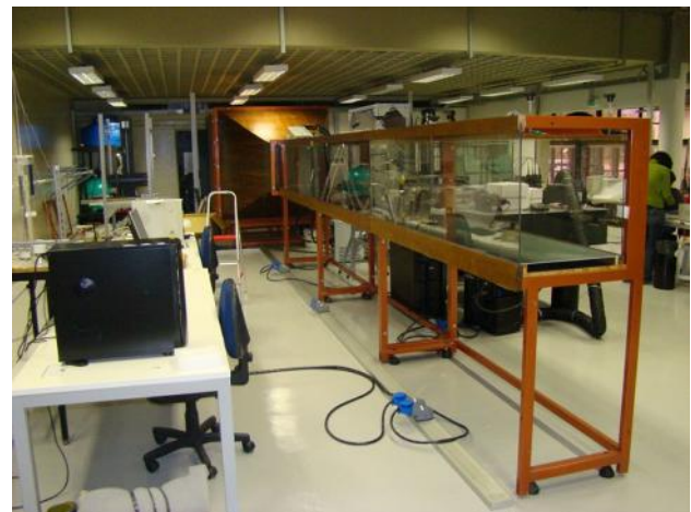
Fig. 5 Open circuit blower-type wind tunnel of DINAM-INMETRO
