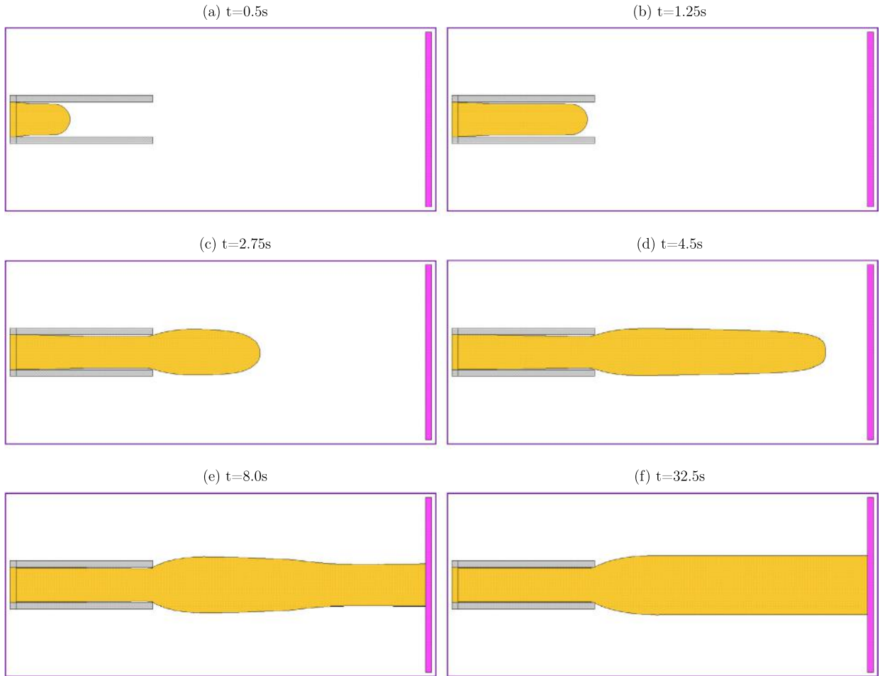
Fig. 14. Numerical simulation of the extrudate swell: fluid flow visualization at different times.
