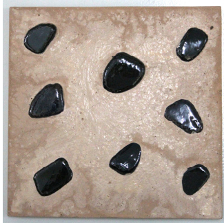
Figure 4. Type III; Tile Body Made of White Portland Cement and 50% of Red Powder, Surface Topping with Artificial Pebbles
