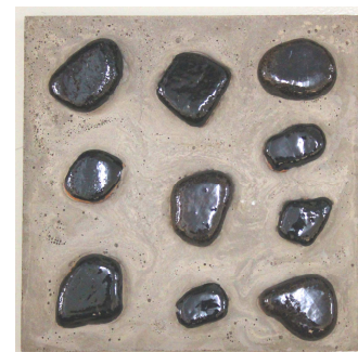
Figure 3. Type II; Tile Body Made of Grey Portland Cement and 10% of Red Powder, Surface Topping with Artificial Pebbles
