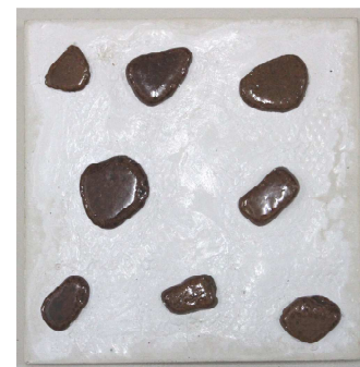
Figure 2. Type I; Tile Body Made of White Portland Cement, Surface Topping with Artificial Pebbles
