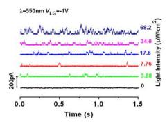
Fig. 4. Drain Current Waveforms at 300 K for Different Levels of Light Intensity at the Wavelength of 550 nm. Baseline Current is Adjusted to 1 nA by  $V_{SUB}$ , and each Waveform is Shifted for Clarity.  $V_D$  and  $V_{LG}$ , are 0.05 and -1 V, Respectively
