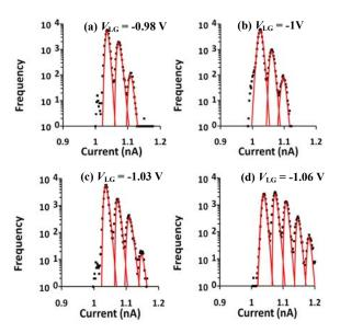
Fig. 7. Histograms of Drain Current for (a)  $V_{LG} = -0.98 \text{ V}$ , (b)  $V_{LG} = -1.00 \text{ V}$ , (c)  $V_{LG} = -1.03 \text{ V}$ , and (d)  $V_{LG} = -1.06 \text{ V}$  with Different  $V_{SUB}$  to Keep the Baseline Drain Current at the Same Level of 1 nA Under the Continuous Light Illumination of 34  $\mu$ W/cm². The First, Second, Third, and Fourth Peaks Correspond to the Number Stored Holes of 0, 1, 2, and 3, Respectively
