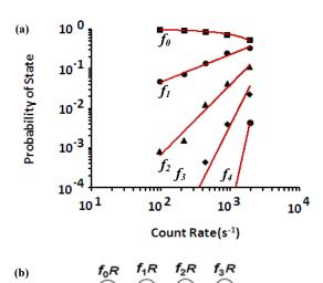
Fig. 6. (a). Probability of States Obtained from Fig. 5 as a Function of Count Rate, Namely, Hole Generation Rate R. State  $f_0$ ,  $f_1$ ,  $f_2$ , and  $f_3$  Correspond to Zero, One, Two and Three Stored Holes, Respectively. (b) State Transition Diagram to Explain (a)
