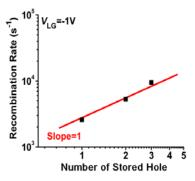
Fig. 8. Hole Recombination Rate as a Function of Number of Stored Holes at  $V_{\rm LG}$ = -1 V. The Data are Derived from the Analysis of the Drain Current Histograms. Slope of the Fitting Line is One
