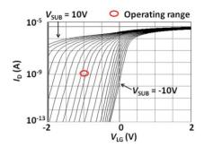
Fig. 2.  $I_{\rm D}\text{-}V_{\rm LG}$  Curve with  $V_{\rm SUB}$  as a Parameter. We Use Bottom Electron Channel and Photo-generated Holes are Stored Below the LG. Drain Voltage  $V_{\rm D}$  is Kept at 50 mV
