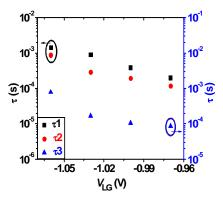
Fig. 9. Hole Lifetime as a Function of  $V_{\rm LG}$ .  $au_1$ ,  $au_2$  and  $au_3$  are the Lifetimes when the Number of the Stored Holes are One, Two and Three, Respectively
