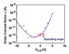
Fig. 3. Noise Evaluation in Dark Condition.  $\sigma$  is the Standard Deviation of the Drain Current for the Bandwidth of 5 Hz.  $V_{\rm LG}$  is Adjusted to Keep the Average Drain Current of 1 nA
