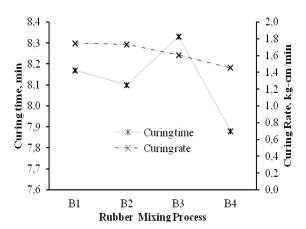
Figure 2. The Curing Rate of and Curing Rate of B under the Rubber Mixing Process Effect at the Vulcanization Temperature of 150  $^{\circ}$ C
