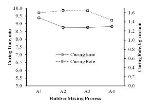
Figure 1. The Curing time and Curing Rate of A under the Rubber Mixing Process Effect at the Vulcanization Temperature of 150  $^{\circ}\text{C}$
