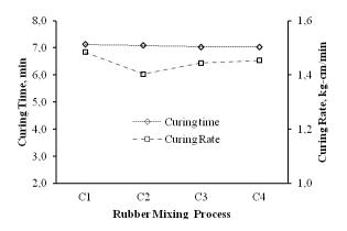
Figure 3. The Curing Rate of and Curing Rate of C under the Rubber Mixing Process Effect at the Vulcanization Temperature of 150  $^{\circ}$ C
