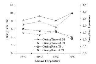
Figure 6. The Curing Time and Curing Rate of B1 and C1 under the Mixing Temperature Effect
