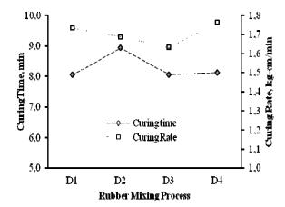
Figure 4. The Curing Rate of and Curing Rate of D under the Rubber Mixing Process Effect at the Vulcanization Temperature of 150  $^{\circ}\mathrm{C}$
