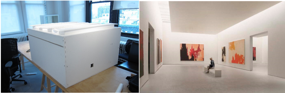
Figure 8: Physical daylight model of gallery: exterior model (left) and interior photograph (right). Source: (Arup 2015)
