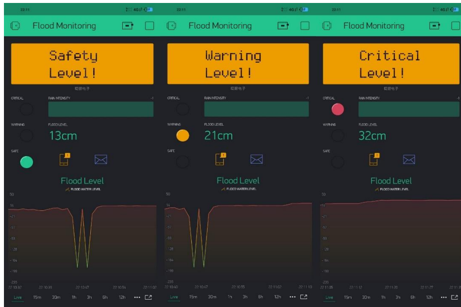
Figure 8. Flood Level Detection Monitoring in Blynk Apps
