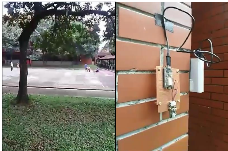
Figure 6. (Left) The actual test bed (an Area between Building E, Building F, and Building G). (Right) The deployment of the End Device at the actual test bed (Sensor Node of Building E)
