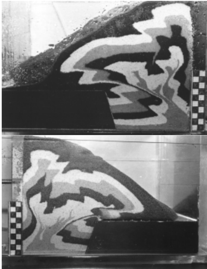
Fig. 6 – Two opposite side wall sections of the same experiment (model M2-a), after 80% shortening, revealing slightly different geometries in the antiformal stack (see text). Scale bar is 5 cm.
