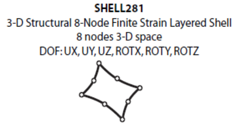
Figure 2. Shell281 as defined in Element Reference ANSYS Release 11.0 (2007)
