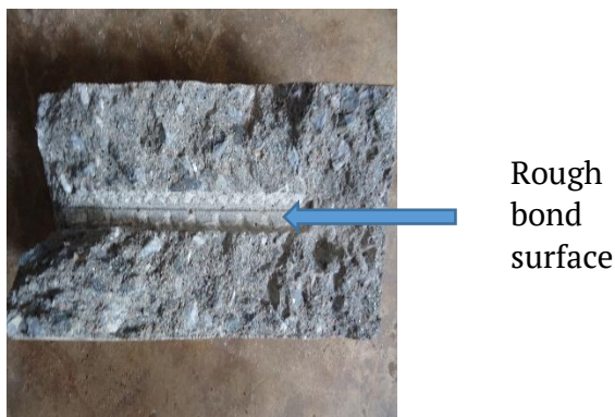
Figure 18. Concrete bond surface (uncoated)
