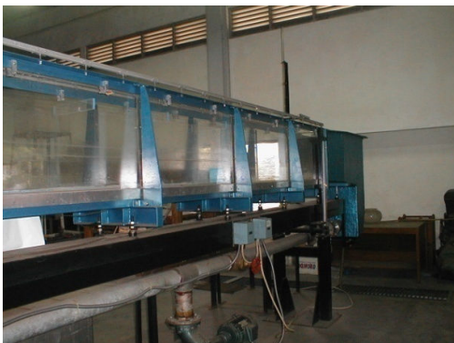
Figure 2. General purpose hydraulics tilting flume
