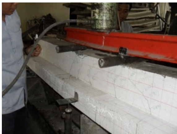
Figure 12. The pattern of crack in the reinforced beam of type 2
