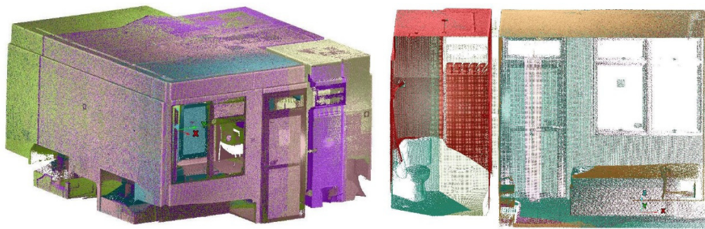
Figure 5. 'Point clouds' processing of outside and inside room with 12.5 mm density
