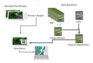
Figure 1. Flow chart of RapMet development (reproduced by permission of Sutrisno et al. 2017)
