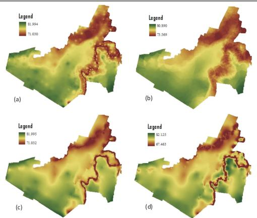
Figure 6. DTM as the Results of (a).IDW Method, (b).Kriging Method, (c).Natural Neighbour Method, (d).Spline Method, (minus 20% validating points)
