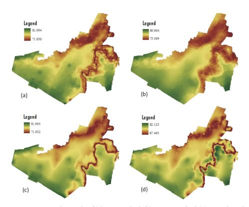
Figure 5. DTM as the Results of (a).IDW Method, (b).Kriging Method, (c).Natural Neighbour Method, (d).Spline Method, (minus 10% Validating Points)
