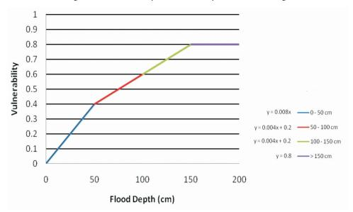
Figure 12. Vulnerability Curve of Paddy at Graining Stage
