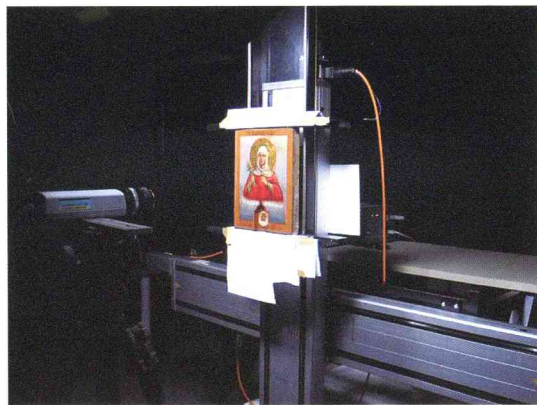
Fig. 5. Spectral imaging system for measuring and digitizing the object.
