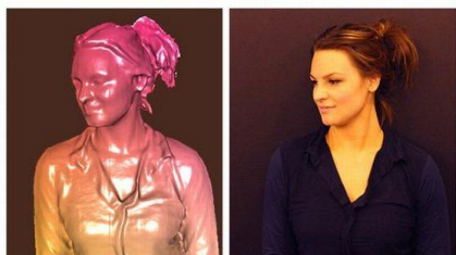
Gambar 2. Contoh Hasil Rekonstruksi 3 Dimensi Kinect (Sumber: https://www.design-engineering.com/3d-freebie-microsofts-kinect-fusion-turns-xbox-controller-into-a-3d-scanner-98643/ )
