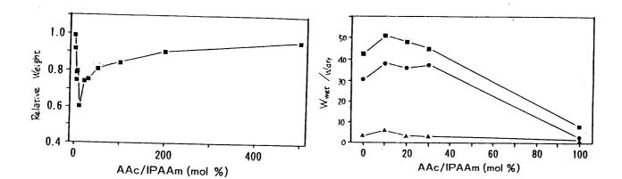
Fig. 1: Effect of copolymer composition on the electrical responsiveness of hydrogel. Electric field: 5V, Time of on-field: 5hrs. AAC/IPAAm: Ratio in mol% of acrylic acid to isopropylacrylamide.
