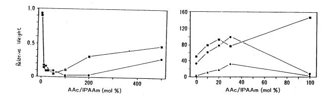
Fig 3: Effect of copolymer composition and hydrolysis time on the electrical responsiveness of hydrogel. Electric field: 5V, 5hrs. Hydrolysis time: 1hr, 4hrs, AAc/IPAAm: Same as in Fig. 1.
