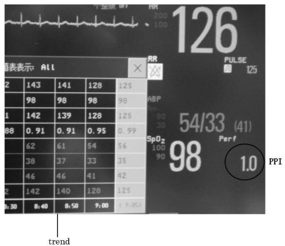
Fig. 1 Actual monitor screen view reflecting PPI and trend values (PHILIPS Intelli Vue MP50)
