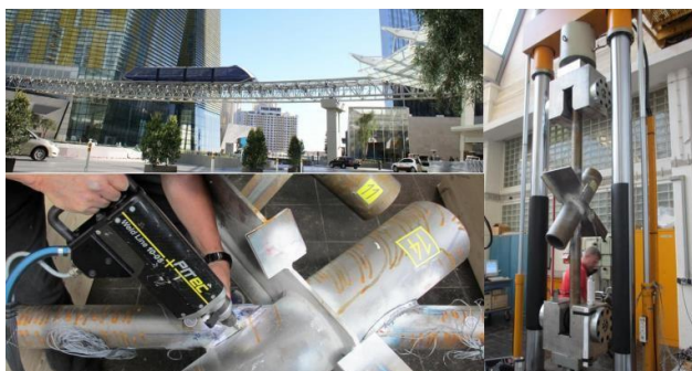
Fig. 17: Application of HFMI/PIT on tubular joint construction.
