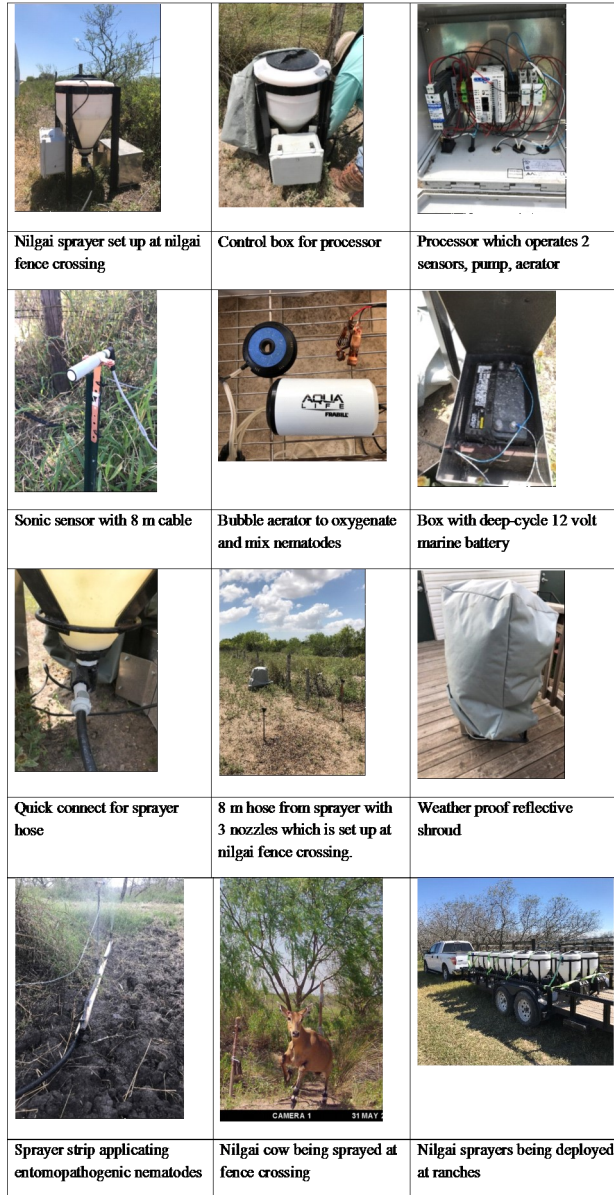
Figure 1. Remotely operated nilgai sprayer
